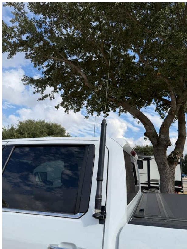
Dave, KS5SK, going over his nice truck install for his dual-band VHF/UHF antenna and his Yaesu ATAS-120A HF antenna.
